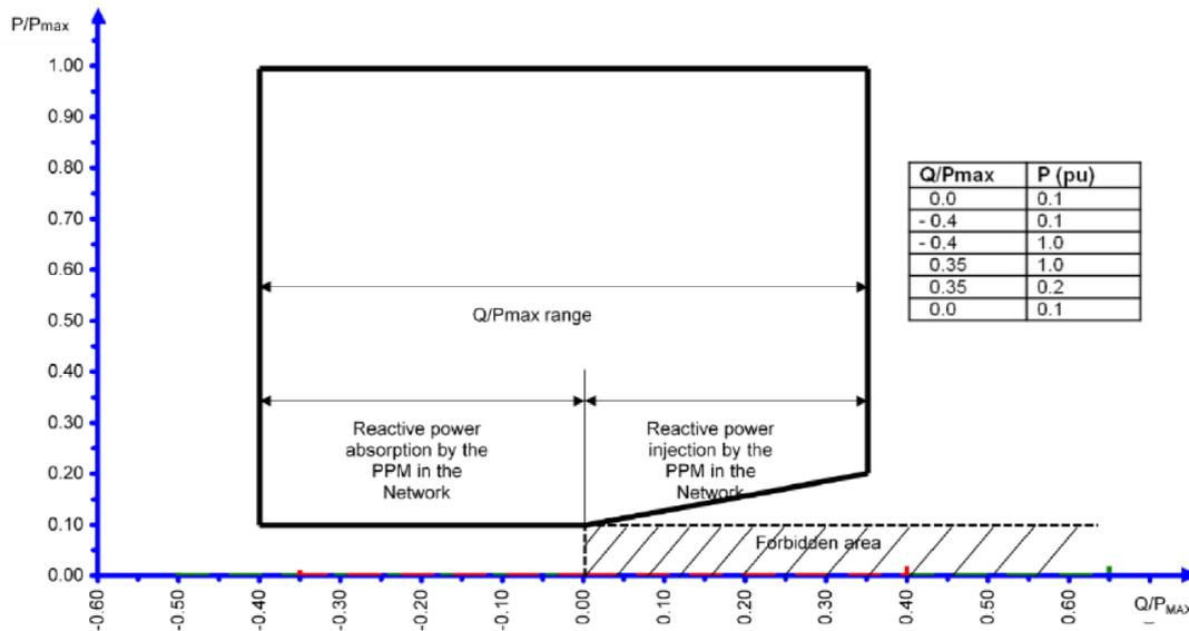
**Figure 1: Reactive power capability acc. SOC 11-175**
