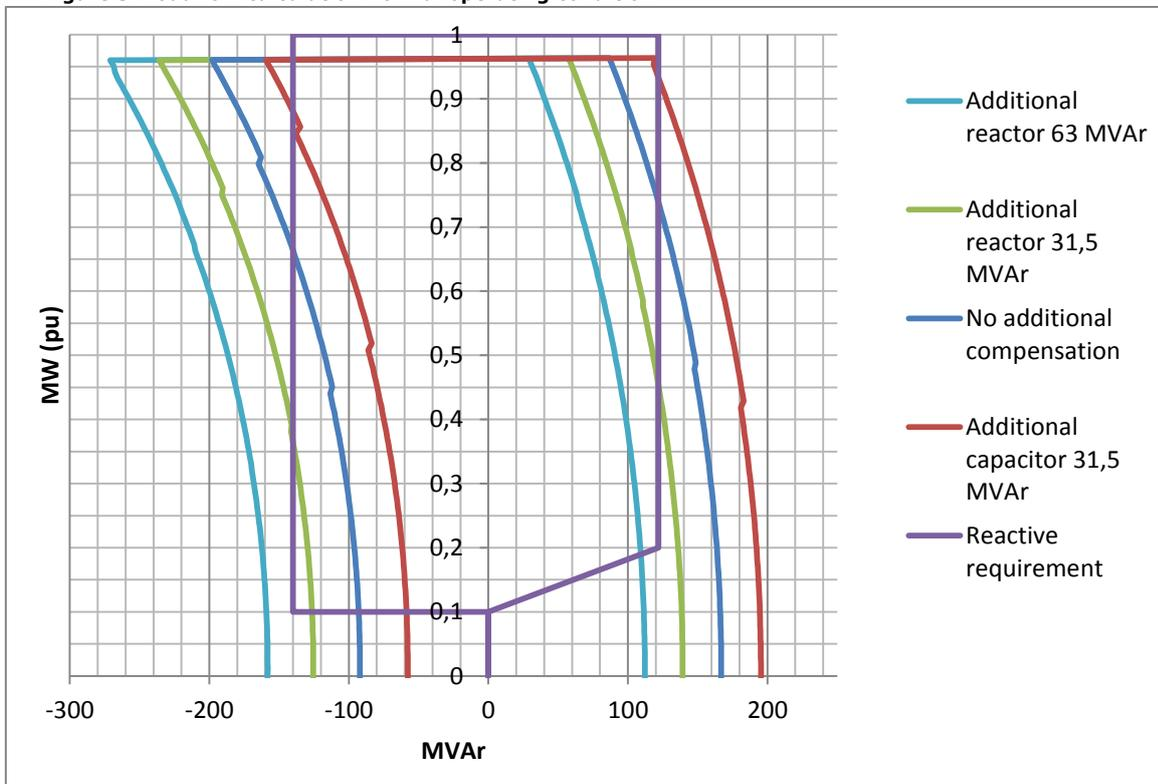
Figure 4: Loadflow calculation extreme reactive power injection/absorption
