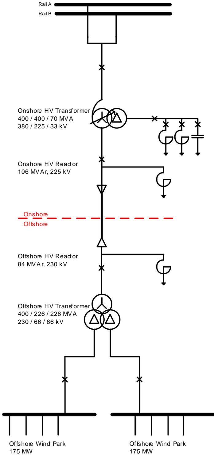
**Figure 2: Single line of grid connection system**
